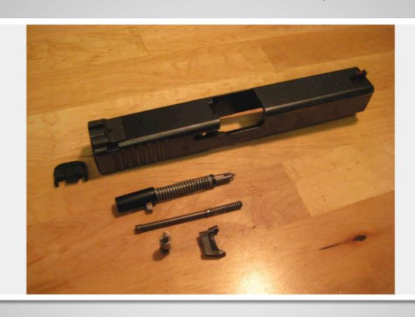
The slide is now disassembled. There is still a liner in the firing pin channel which generally does not get replaced. Your slide is now fully disassembled. Now you can move on to replacing the firing pin spring.
