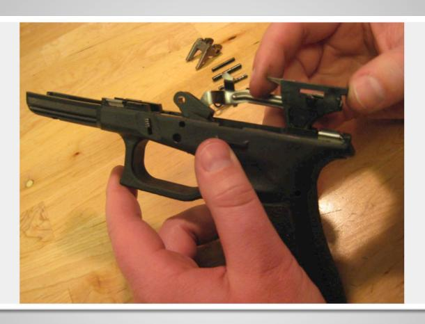
Place the trigger group back into the frame. Replace the locking block, slide stop lever and pins and you have a completely assembled frame. Insert barrel and recoil spring into slide and attach slide to frame. Your Glock pistol is now completely assembled.
