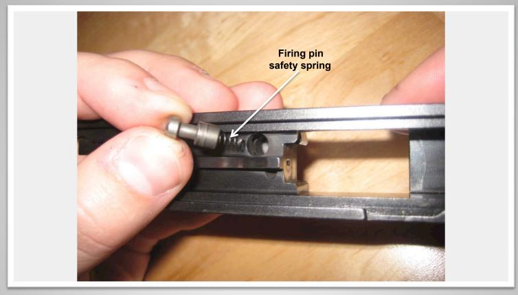
Remove the firing pin safety and firing pin safety spring from the slide. This is also a step where you can replace the firing pin safety spring in the firing pin safety. Insert the spring in to the bottom area of the firing pin safety push and twist (counter clockwise) until it is seated. IMPORTANT:
