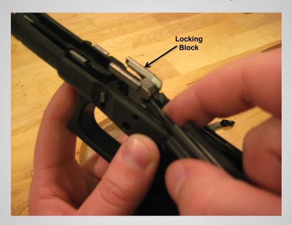
Gently pry the locking block out of the frame. These can be very tight in a new gun.
