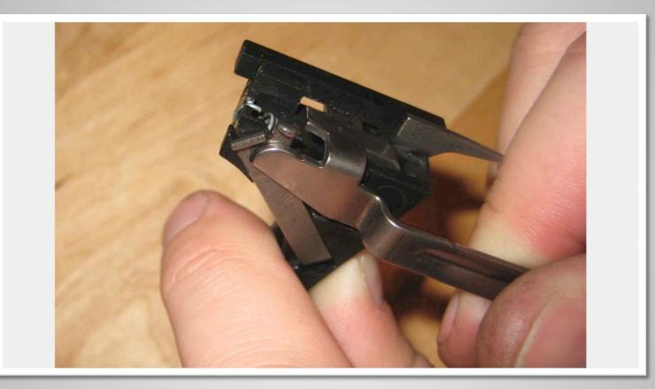
Finally rotate the cruciform into the channel on the high side of the trigger housing and release. You have successfully assembled the trigger group.
