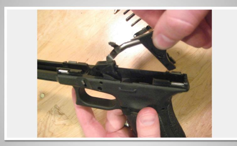
Grab the trigger housing on both sides and simply pull the trigger assembly out of the frame.
