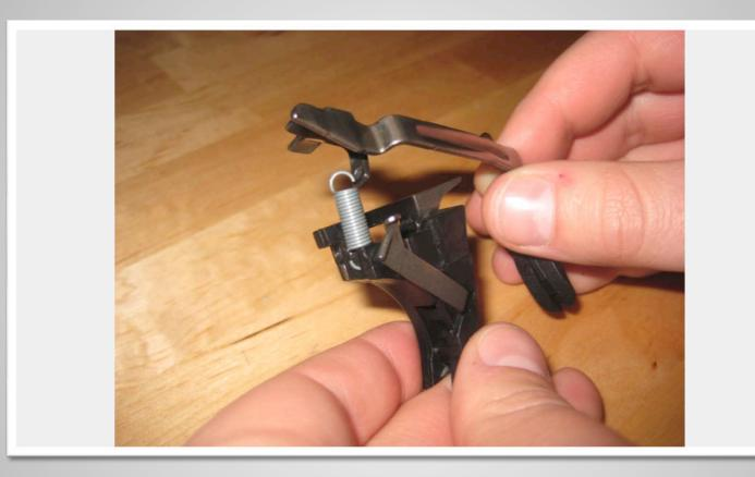
The hook part of the spring will be inserted through the hole in the trigger bars trigger spring arm.
