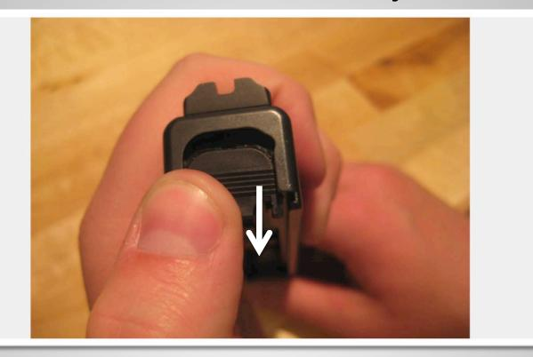
**WARNING!** The extractor spring assembly can "shoot out" of the slide during this step. Great care should be exercised and eye protection worn!
