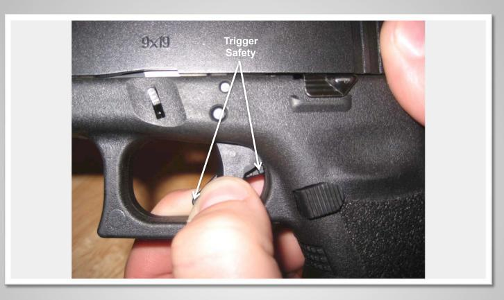
With your Glock re-assembled, check to make sure it is "UNLOADED". With the gun pointed in a "Safe Direction" grab both sides of the trigger, making sure not to depress the trigger safety. Push the trigger toward the rear of the trigger guard. A functional trigger safety will hit the frame and stop the gun from disengaging (dry firing).
