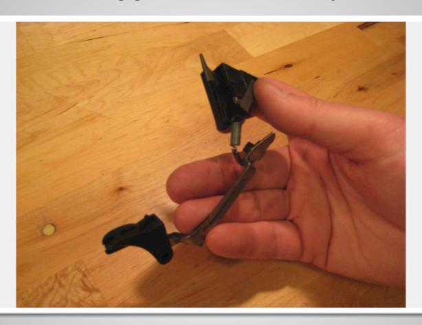
You have now disconnected the trigger w/ trigger bar from the trigger housing. Now remove the trigger bar from the spring.
