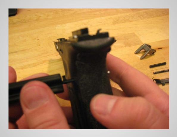
Push out the trigger housing pin.
