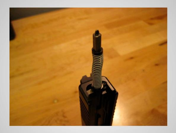
To remove the spring cups and replace the firing pin spring, place the assembled firing pin (with spring, spring cups, and spacer sleeve) into the slide (firing pin channel) with the firing pin lug turned and resting where the slide cover plate is when installed.
