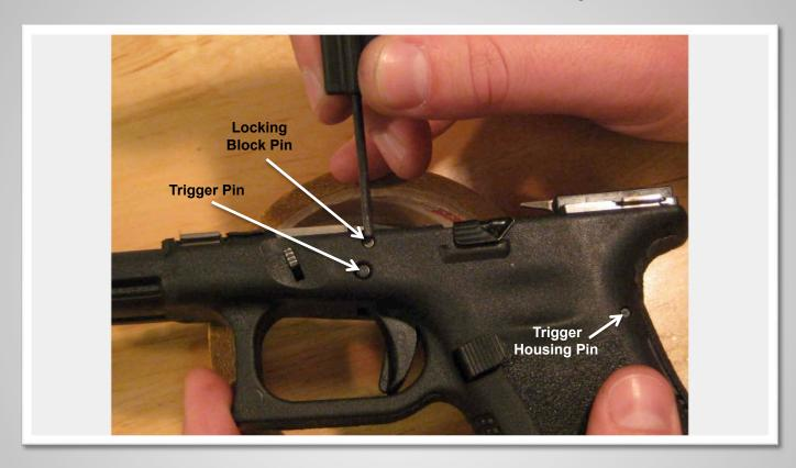
Push the locking block pin all the way through the frame until it drops out. This pin may not be present on some earlier models (some models had only 2 pins).
