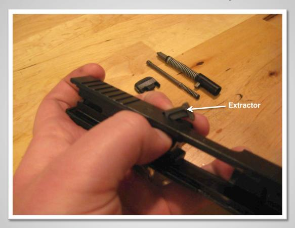
With the firing pin safety fully depressed from the last step, rotate the extractor out of the slide.
