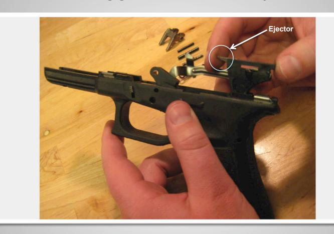
Gently lift the trigger housing by pulling up underneath the ejector.
