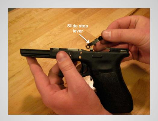
The slide stop lever is now free and can be removed. NOTE: When re-assembling, the slide stop lever must be installed after the locking block pin. Insert the lever with the spring facing upward and slide it into the first groove on the left side of the frame. Gently push forward and hold in place while pushing the trigger pin through the frame. You will most likely need to "wiggle" the slide stop lever to allow the trigger pin to pass through.
