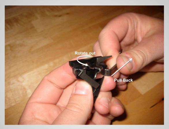
Hold the trigger housing in one hand and the trigger bar (behind the trigger tab) in the other. Pull the trigger bar straight back toward the ejector end of the trigger housing when the cruciform (cross shaped) part of the trigger bar hits the inside of the trigger housing then rotate out and away from the housing.
