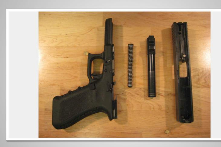
You will need a Glock disassembly tool or a 3/32" punch, to take apart your pistol completely.
