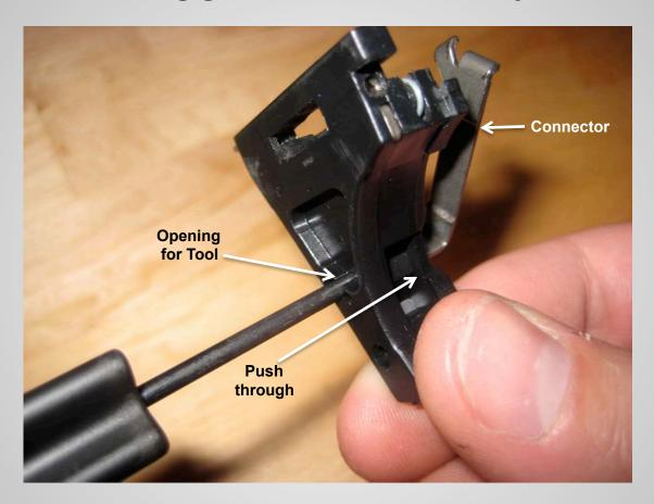
Next push the connector all the way out of the trigger housing from the opposite side.
