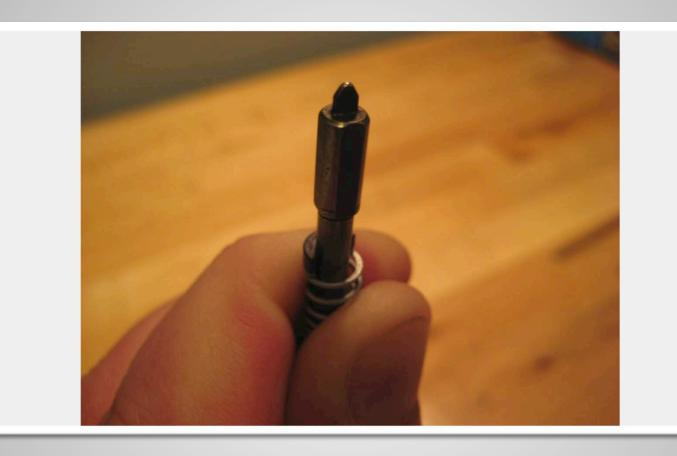
Replace the spring cups: This can be difficult; grasp the spring firmly in the middle of the spring, and pull down until there is enough clear space on the striker to replace the spring cups. Make sure the spring cups fit together flush and the thinner ends are inside of the spring.
