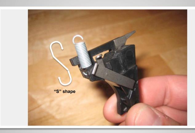
The open end of the "S" shape made by the trigger spring faces forward toward the ejector. The trigger spring should always be installed with this same "S" shaped configuration.
