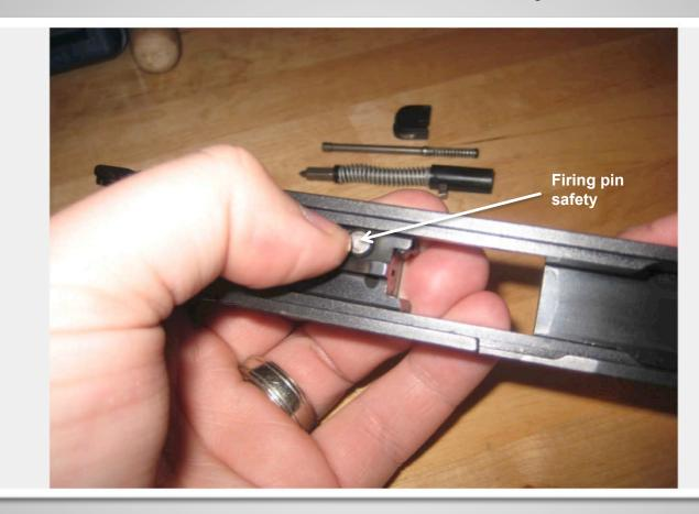
Depress and hold the small, round, silver-colored button (firing pin safety) on the bottom of the slide as shown. Keep the firing pin safety depressed during the next step.
