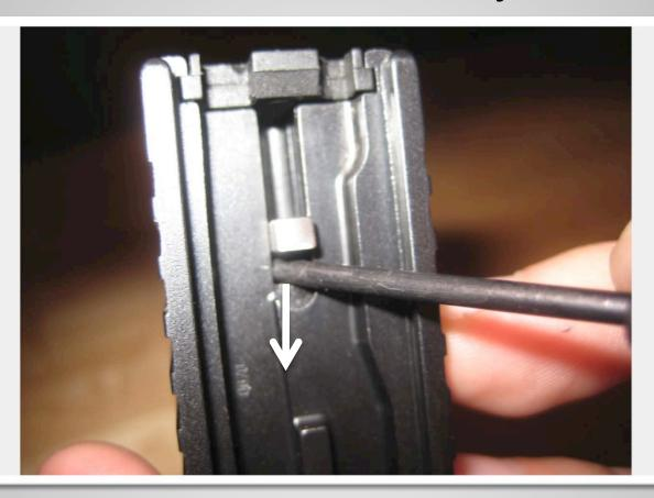
Using a disassembly tool push down the polymer spacer sleeve as shown. Hold the sleeve down for the next step.
