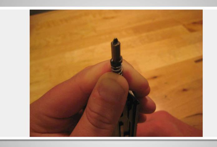
Slowly release tension on the spring until the spring cups are pressed against the thicker portion of the striker. *Re-assemble* the slide and all of it's parts, by reviewing the previous steps. You now have completed the steps necessary to to upgrade the slide assembly. Before you move on to the frame upgrade, we will do a "safety check" on the slide assembly.
