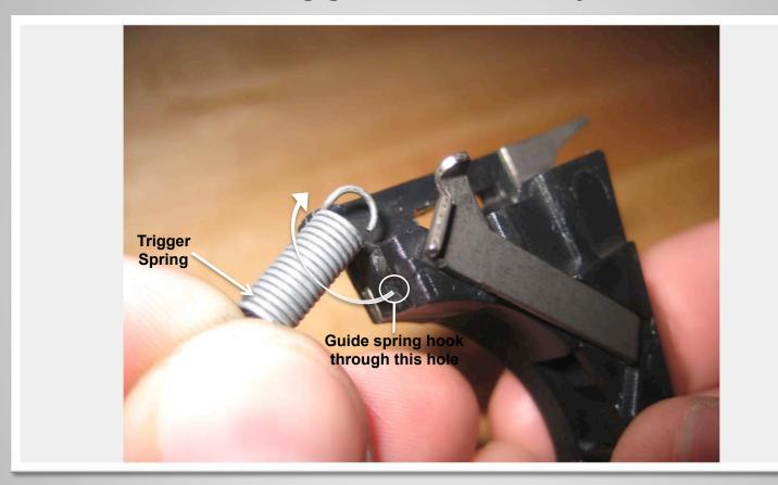
Push the connector back into the trigger housing. Insert the trigger spring open end down (as shown). The spring goes over the back lip of the housing and threads through the hole below the small notch. Then rotate upward.
