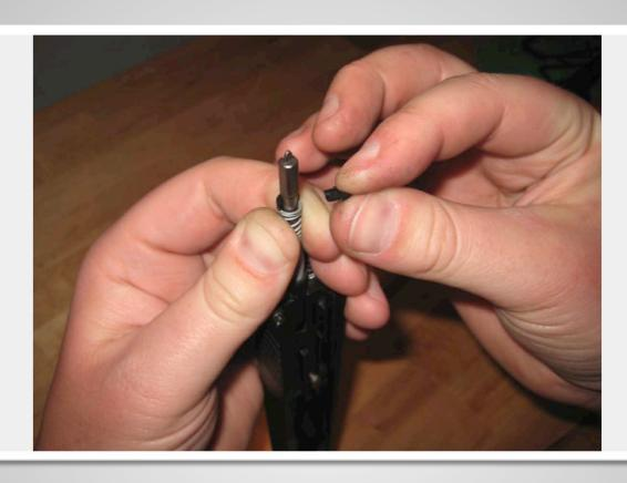
Wrap your hand around the slide for support while pulling down on the firing pin spring remove each ½ of the spring cup set. (CAUTION: These spring cups and spring can fly off and possibly cause eye injury, make sure to wear safety glasses).
