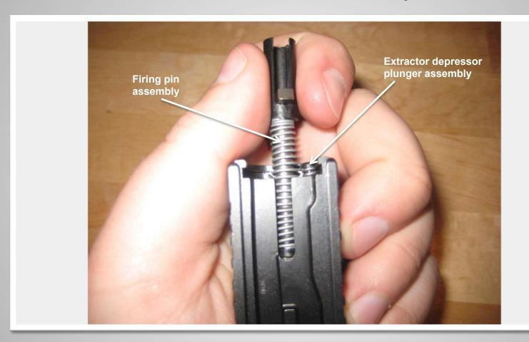
Remove the firing pin assembly and extractor depressor plunger assembly.
