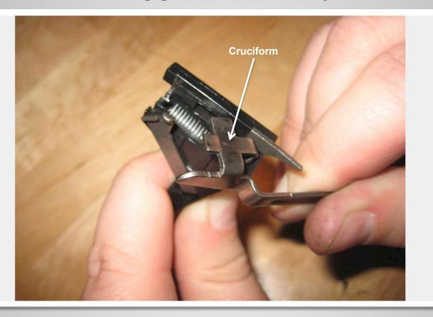
When the spring is attached pull the trigger bar back at an angle turned outward and drop the spring arm into the housing.
