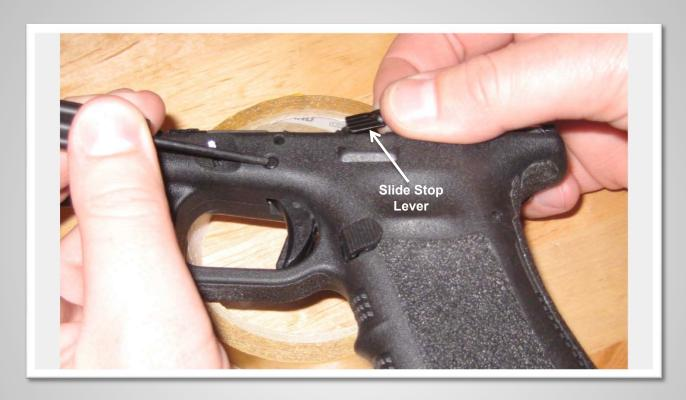
The slide stop lever is spring loaded into a groove in the trigger pin. Slowly "wiggle" (up & down and front to back) the slide stop lever while pushing on the trigger pin until you can feel the trigger pin start to move. Do not apply excessive force, keep manipulating the slide stop until the pin moves. Then push the trigger pin out of the frame.
